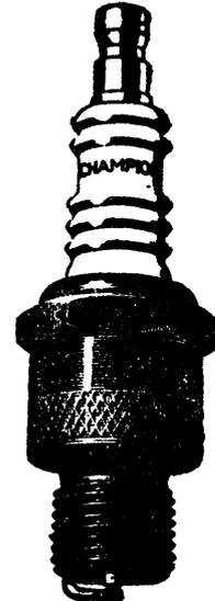
*Fig. 3. The sparking plug*
