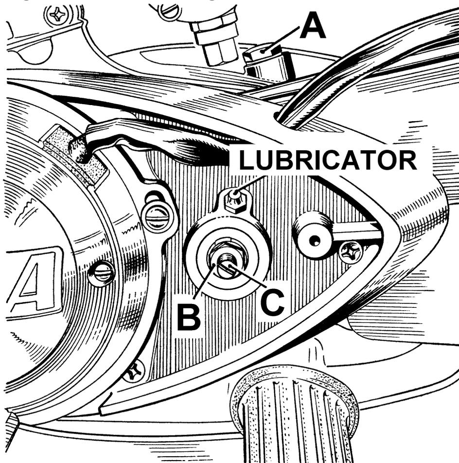
*Fig. 6. Clutch control adjustment, with outer cover removed.*
