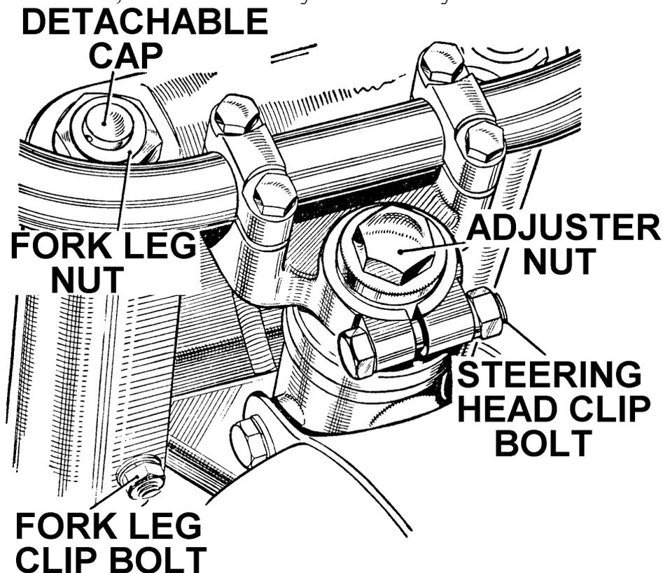
*Fig. 8. Front Fork and steering head*
